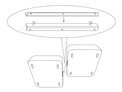
Lift the aligned modules so that one connector engages the other and carefully lower the already engaged modules.
