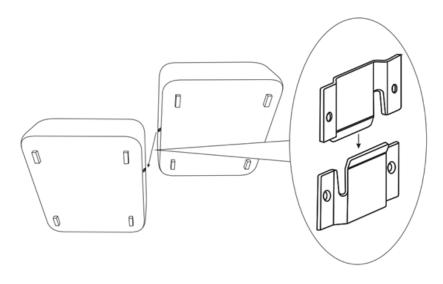
Lift one of the aligned modules so that one connector fits into the other and carefully lower the already engaged module.
