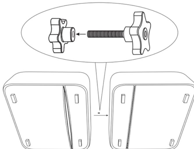
Thread the handle onto the screw to connect the two modules and close the zipper.
