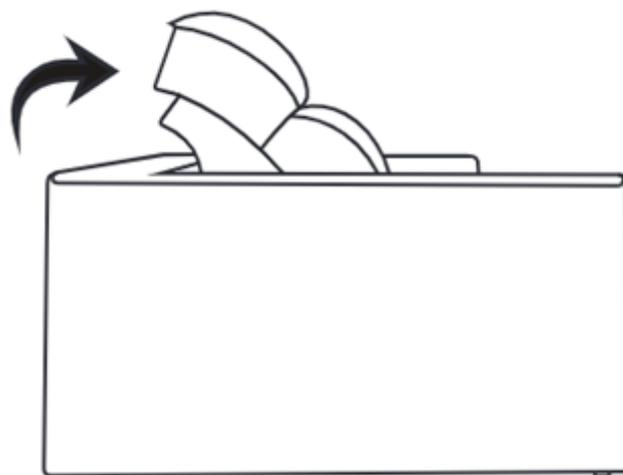
**Step 2:** To unlock, push the backrest all the way down, as indicated by the arrow, and return to the horizontal position.
