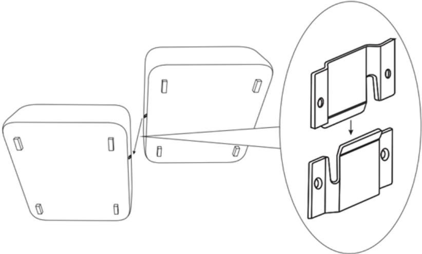
Lift one of the aligned modules so that one connector fits into the other and carefully lower the already engaged module.
