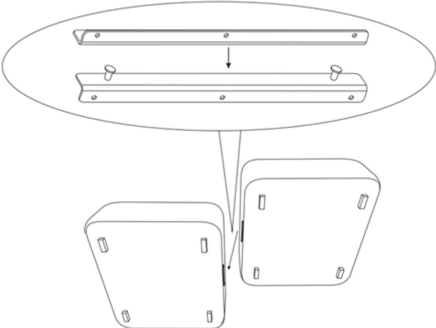
Lift the aligned modules so that one connector engages the other and carefully lower the already engaged modules.
